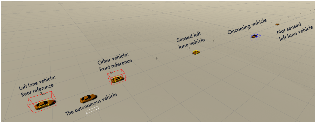
Figure 4: The simulator view. AV is overtaking two consecutive vehicles. Vehicles with yellow boxes around them are sensed by the 360-degree sensor. Vehicles with red boxes around them are used as reference points for the acceleration and braking manoeuvres. OV , marked with a blue box, is sensed using the long range sensor.
