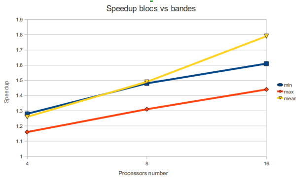
Figure 6: The speed-up obtained by reading single blocks compared to reading 16-block bands.
