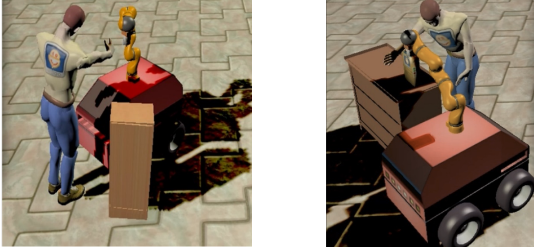
(a) Morse output for a single time instant, where the gripper of the robot and human arm are very close but an actual contact has not happened. (b) Morse output for another time instant, where model checker and simulator both detect a hazardous contact between human arm and the gripper of the robot.
