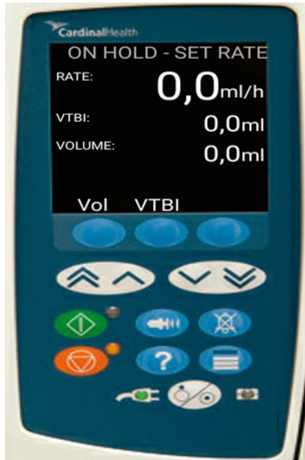
Figure 4: Front panel of the Alaris GP infusion pump.
